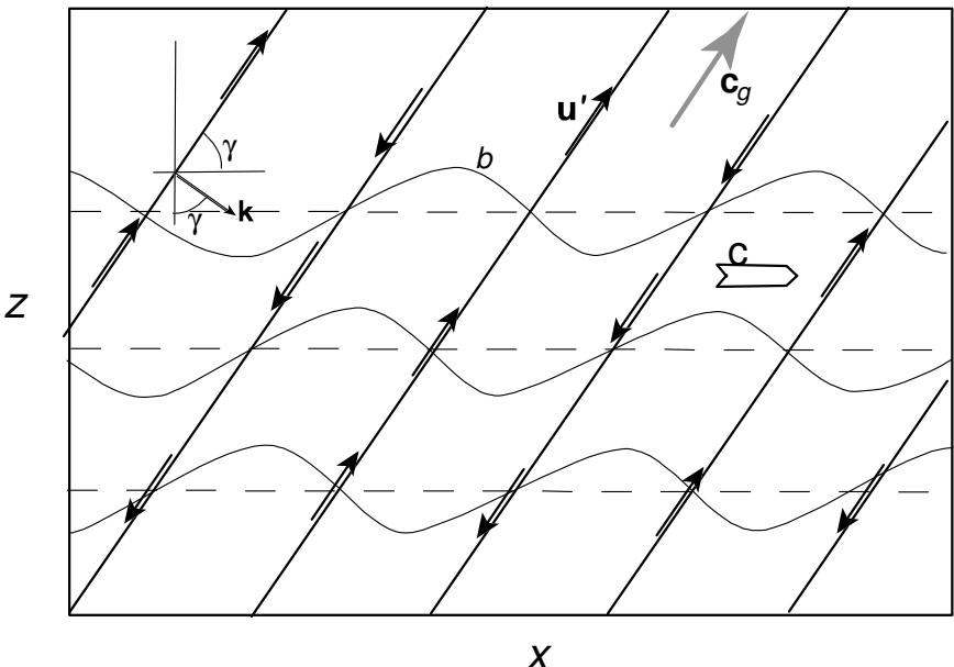
From localized source of frequency  $\omega$ , waves form rays at angles  $\gamma = \sin^{-1}(\omega/N)$  to horizontal, with phase propagation *across* rays:
